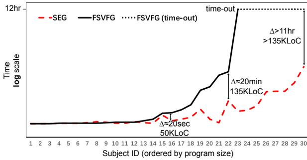
Figure 7. Time cost: building SEG vs. building FSVFG.
