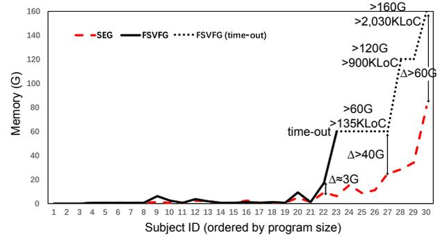
Figure 8. Memory cost: building SEG vs. building FSVFG.
